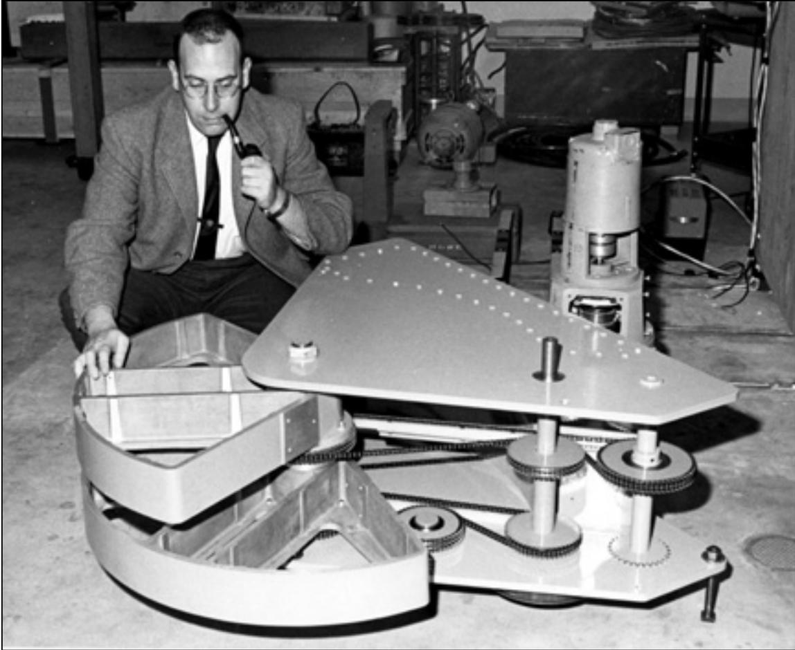
This earthquake-making instrument was part of a project sponsored by the Earthquake Engineering Research Institute under the direction of George W. Housner and Donald Hudson. The machine weighs close to 500 pounds, including its 1.5 horsepower motor. Shaking is produced by a pair of 20-inch swing boxes that counter-rotate unbalanced amounts of lead weights. The machine was designed by Dino Morelli, while Thomas Caughey developed the electrical design. Photo by James McClanahan, 1959.
