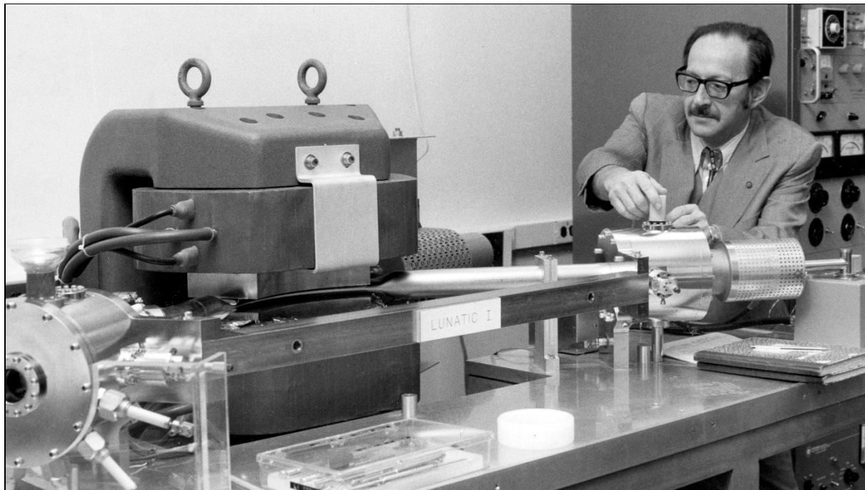
Wasserburg with Lunatic I, the first fully digital mass spectrometer with computer-controlled magnetic field scanning and rapid switching. Donated to the National Museum of American History in 2009. (Photo taken in Wasserburg's lab at Caltech in 1978.)
