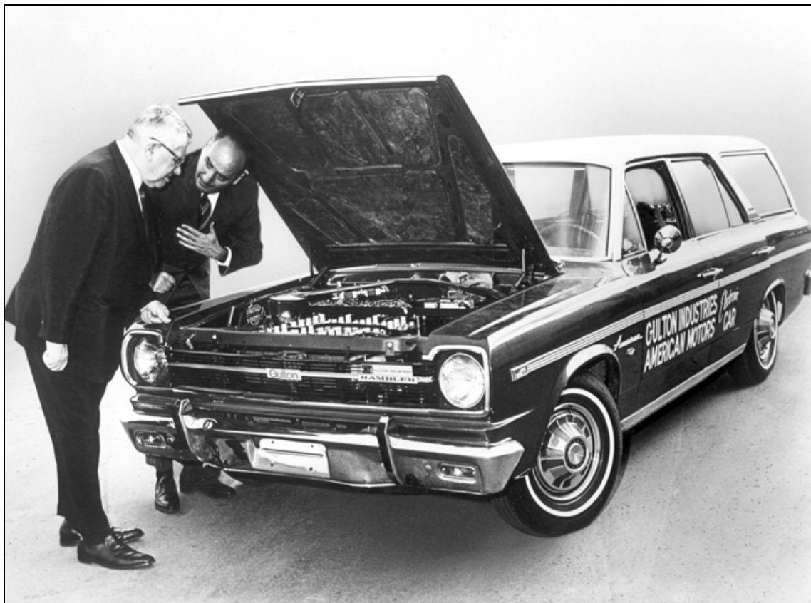
Fig. 4. Wouk explains to Congressman Edward Patten the function of the nickel-cadmium batteries in the power system of the Gulton-American Motors electric car in November 1969. Caltech Archives.
